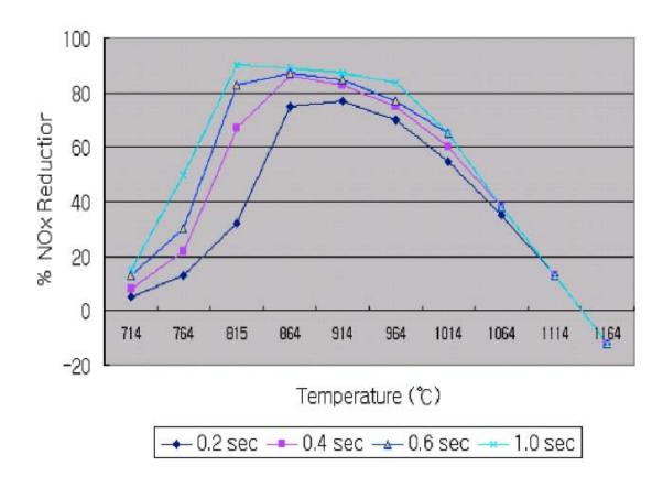
The reagents needs to be injected in a ideal temperature range of 900-1050 °C.
