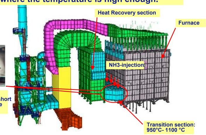
The SGM achieves high quality mixing in a very short space and a low pressure drop (about 1mbar).
